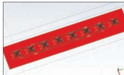
▲ Fig. 3 Modeled eight-element single tier elevation array.
