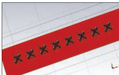
▲ Fig. 6 Modeled single tier azimuth array.
