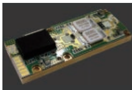
S-Band 250W 30dB Gain, 20% DC, 1mS PW in (7.5cm x 3cm)
