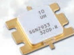
50 \Omega Matched 2.9 - 3.3 GHz Gp = 13 dB 320 W
